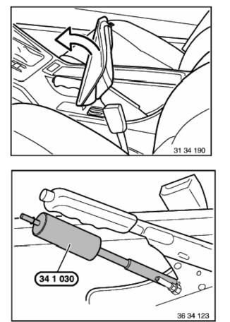
Lift out dust cover. Remove tunnel tray, refer to Gr. 51
