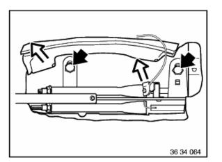
Unscrew bolts. Remove handbrake lever.
